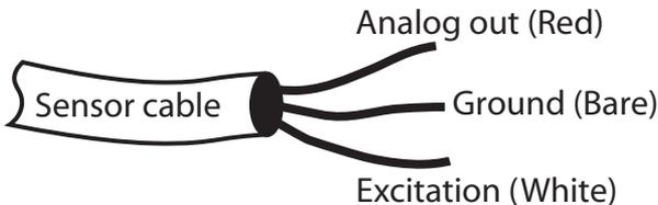
10HS sensors with the stripped and tinned cable option can be made with custom cable lengths (up to 250 ft) on a per-foot fee basis. This option gets around the need for splicing wire (a possible failure point).
