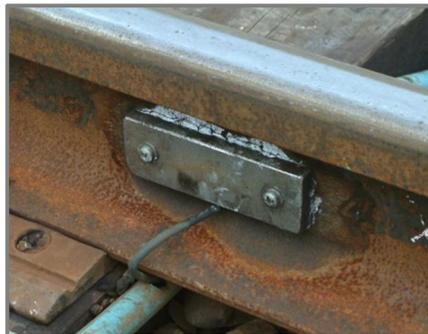
Figure 1 - Track Temperature Sensor
